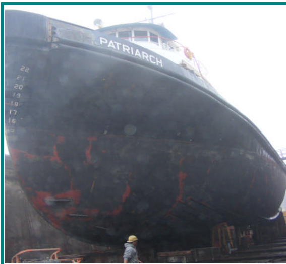
Prior to surface preparation and coatings
