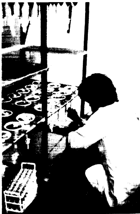
Figure 2. Technician collecting sediment from funnels. Funnel stand showing construction of the racks to support funnels, the funnels with clamps and splash trays. 80 samples could be tested in a stand like this.
