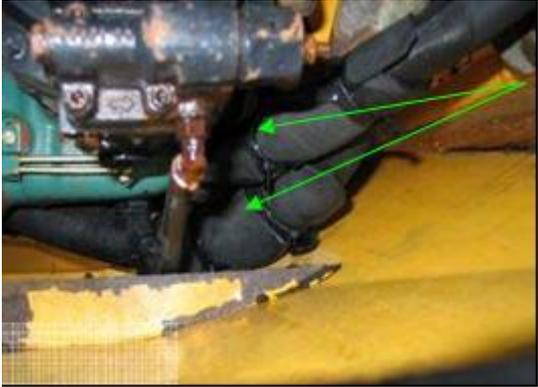
A close-up photograph of hydraulic hoses. Two green arrows point to black foam insulation that is wrapped around the hoses.                                                                                                 |
