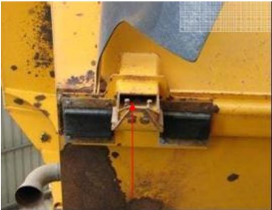
A close-up photograph of a hollow channel under a yellow metal tray. A red arrow points to the channel, which is filled with dark, contaminated grease. A white pipe is visible in the background.                                      |
