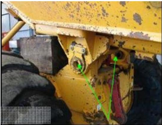
A close-up photograph of a yellow machine's pivot point. Two green arrows point to the pivot joints, which are heavily greased. A red pipe is visible in the background.                                                                 |
