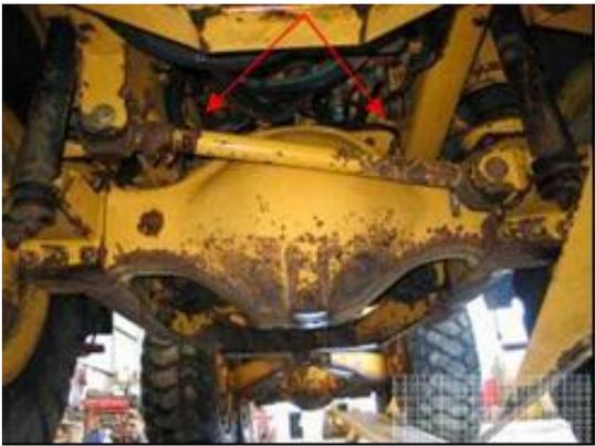
A photograph of the underside of a truck chassis, showing the differential and other mechanical parts. Two red arrows point to the topside of the differential housing.                                                     |
