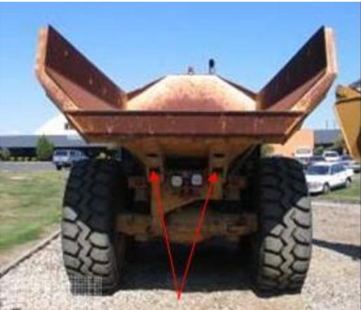
A photograph showing the rear view of a large, rusted dump truck. The dump tray is lowered. Two red arrows point to the exhaust openings located on the rear of the chassis, below the tray.                                                       |
