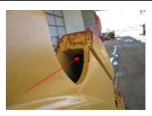
A view of this boot reveals that it is not completely sealed (only spot welded) in place. The green arrow highlights the small recesses, allowing contaminants inside this hollow cavity (blue arrow). These will require further investigation to verify cleanliness. Flushing via these small recesses with a pin jet, will not suffice in removing BRM or verifying internal cleanliness. All boots must be removed (illustrated in second image). Once removed, access is easy for verifying (red arrow).
