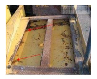
The left and right hand side of the compactor, just in front of the rear drums. On this model there are no non-affixed panels, allowing sufficient access to the side of the engine block for cleaning and inspection. On other models, non-affixed panels will need to be removed to allow this access.
