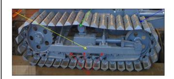
The hollow track frame highlighted previously, may have drainage holes (red arrows) at the end or along the bottom – see next illustration. Pieces of cork have been placed in these holes, however they still require flushing.
