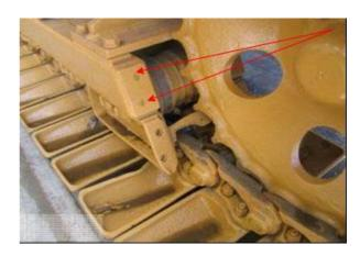
Another way to access the hollow track frame is via the bolt holes (blue arrow) after the rock guards have been removed. Small recesses (green arrow) also require inspection. Flush around the perimeter of the roller (yellow arrow) to verify cleanliness.
