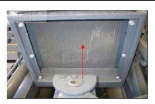
The belly plate has been removed, allowing cleaning and inspection access to the underside of the radiator (red arrow). All ledges (green arrow), hoses (yellow arrow) and the underside surface of the sump (blue arrow) must be cleaned and free of all BRM.
