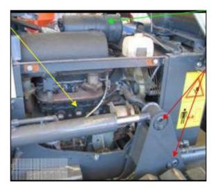
The left hand side of the block. The engine cover and side panels have been removed to allow access for cleaning and inspection. The hydraulic rams and pivot points (red arrows) must have all contaminated grease removed. All surfaces of the block (yellow arrow), including oil filters (blue arrow) and hoses (green arrow) must be thoroughly cleaned and inspected.
