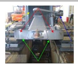
The front of the radiator core. The radiator fins must be flushed to verify cleanliness (red arrow).
