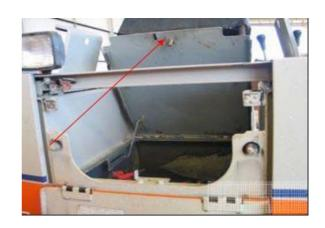
The batteries (green arrows) must be loosened from the tie down points to allow cleaning and inspection of the underside. All internal surfaces must be clean and free of all BRM (blue arrow).
