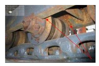
Inside some track frames, V-shaped channels like the one illustrated may be present (yellow arrow). These may be sealed units however they must be verified clean if open from the topside or only spot welded in place.
