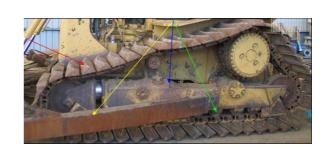
To enable thorough cleaning and inspection, all rock or stone guards (green arrows) which are commonly found on smaller model dozers, must be removed.
