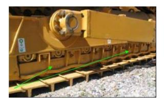
On other small models the topside of the track frame may have numerous non-affixed panels (green arrows) which all must be removed for cleaning and inspection.
