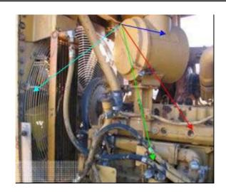
The right hand side of the block also highlighting the side of the block (red arrow), hydraulic hoses (green arrow) and part of the engine housing (blue arrow) which must be checked for hollow or openended channels.
