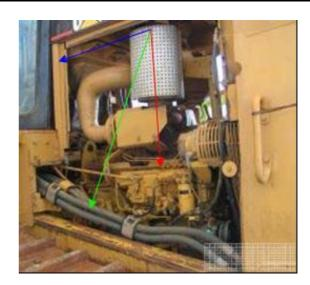
The underside of the block of a medium sized dozer. The belly plates have been removed, allowing cleaning access to the sump (red arrow), engine mounts (blue arrows), hydraulic hoses (green arrows) and harmonic balancer (aqua arrow).
