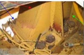
Some ROPS have large recesses underneath and can be full of biosecurity risk material as highlighted by the red arrow.
