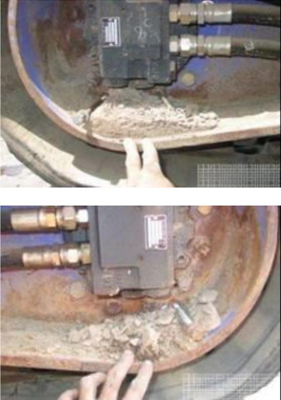
Two photographs showing the interior of a motor cover. The top photo shows a hand reaching into a motor housing where a pile of light-colored, fibrous material is visible. The bottom photo shows a similar scene with a hand reaching into a motor housing containing a pile of light-colored, chunky material. |
