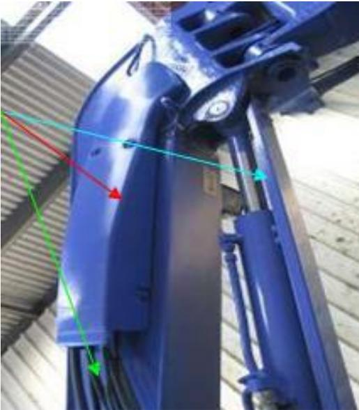
A close-up photograph of a boom stick with several components. A red arrow points to a non-affixed panel, a green arrow points to a hydraulic hose, and an aqua arrow points to a protective plate. |
