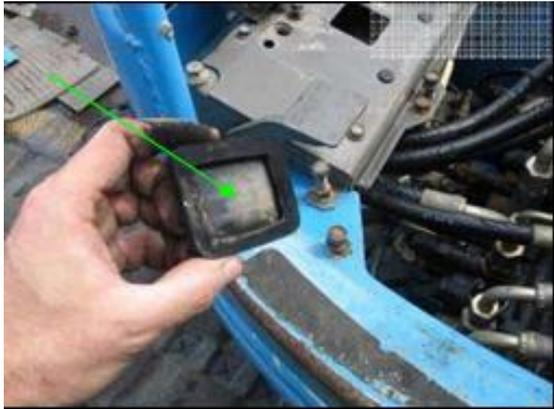
A close-up photograph showing a person's hand holding a black, rectangular foot pedal. A green arrow points from the top-left corner of the pedal towards the center. The pedal is being held in front of a blue metal component of the excavator's chassis. |
