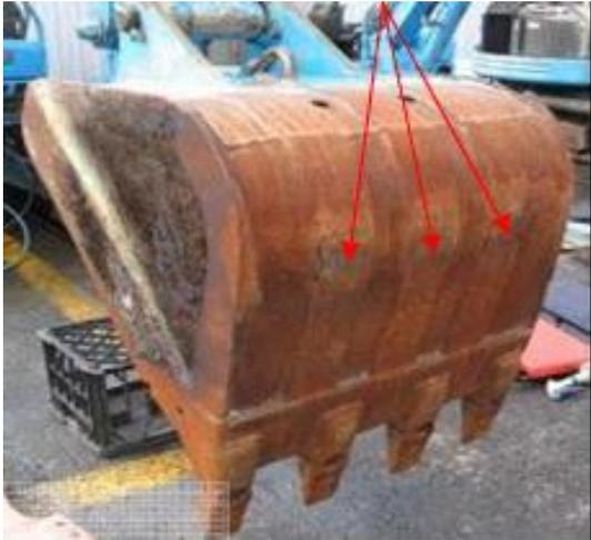
A large, rusted metal bucket is shown from a side-on perspective. Three red arrows point to the bottom edge of the bucket, highlighting the area where wear plates are located. The bucket is outdoors, and a black plastic crate is visible in the background. |
