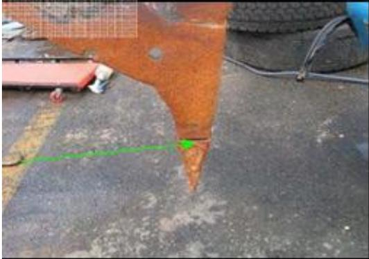
A close-up view of a sharp, pointed cutting tooth on the bucket. A green arrow points to the tip of the tooth. The background shows a dark, textured surface, likely the ground or a workbench.                                                                |
