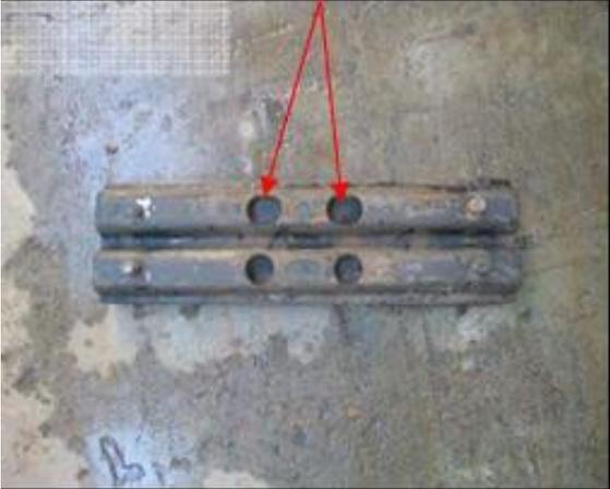
A close-up photograph of two parallel metal track links. Two red arrows point downwards from the top of the links to the small circular recesses between them, showing where biosecurity risk material can be compacted.                                                                                           |
