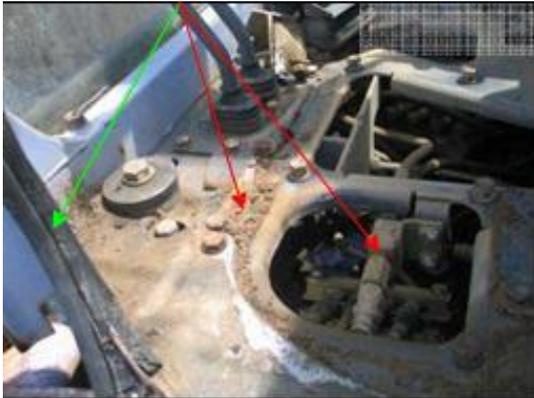
A close-up photograph of the engine compartment of a mini excavator. A green arrow points to a rubber seal on the left side of the engine housing. Two red arrows point to dark, oily residue on the engine components and a circular opening on the right side.                                                                                                                                                                                |
