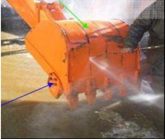
A person is using a high-pressure water hose to flush the bucket. A green arrow points to a spot-welded wear plate on the bottom of the bucket, and a blue arrow points to a side wear plate. The bucket is orange, and the water spray is visible.           |
