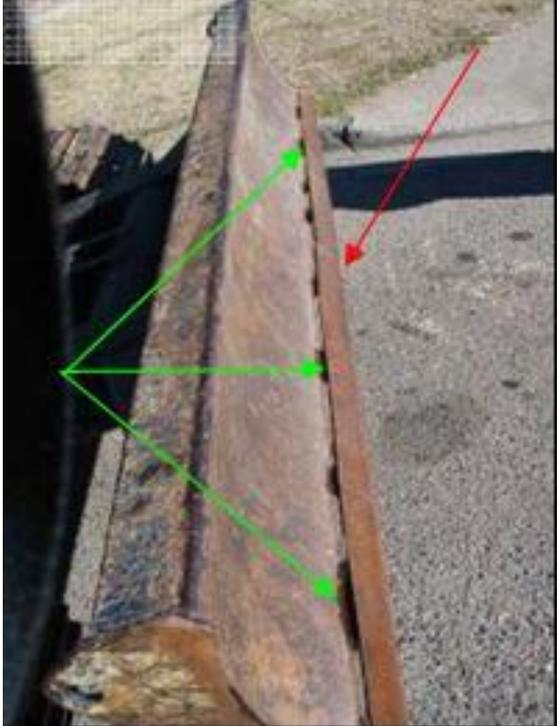
A close-up photograph of a rusty, weathered metal blade. A red arrow points to a small, dark spot weld on the blade's surface. Three green arrows point to various recessed areas along the length of the blade, indicating areas that need to be flushed for cleanliness. |
