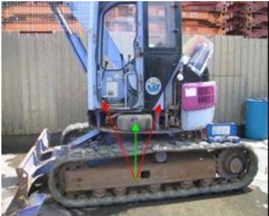
A photograph of a mini excavator with its cabin removed. Red arrows point to drainage holes on the underside of the chassis. A green arrow points to the underside shroud. The hydraulic system and other components are visible under the floorpan. |
