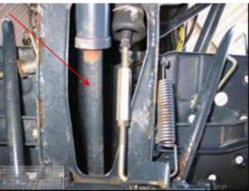
Small recesses like the one highlighted (red arrows) will require flushing to remove any biosecurity risk material and to verify cleanliness.
