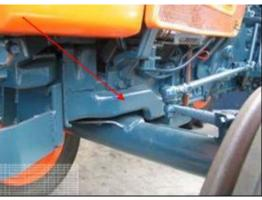
Although not visible in these illustrations, the access points to the hollow channels mentioned above are highlighted by the red arrows. The green arrows indicate the direction of the hollow channel.
