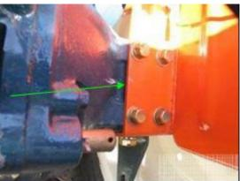
Check for any biosecurity risk material in areas where attachments are mounted to the rear of the tractor (red arrow). Areas like those illustrated by the red arrows may require flushing to verify cleanliness.
