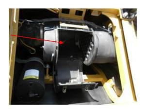
The batteries (red arrow) are to be loosened from the tie-down points and inspected underneath. In newer scrapers the batteries are located under the front of the cab, removing the cover to allow access also allows access to the hollow sections of the front draw bar.
