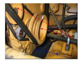
The radiator grill has been removed, allowing inspection access into the bottom of the shroud.
