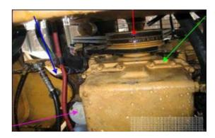
The left hand side of the engine block. Check all the engine cover panels for open-ended or spot welded hollow supports (red arrows), which will require flushing. Check each hydraulic hose, wiring harness and engine mounts (blue arrow).
