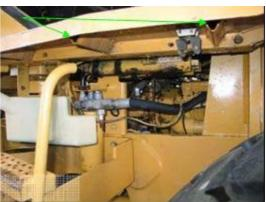
Note that the counterweights have been removed from the rear drawbar (red arrows). The area highlighted by the blue line is hollow and access will be shown next.
