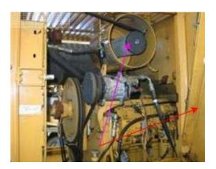
Illustrates the rear of the wheel loader and the radiator grill open, exposing the oil cooler and radiator fins (red arrows), which need to be flushed in the presence of the inspecting officer in order to verify cleanliness. Check all internal surfaces of the light covers (blue arrows).
