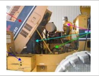
This picture illustrates the side of the engine block and the air-filter housing, which has had the outer filter removed (purple arrow). On this particular model the engine cover is accessed, by opening hinged doors (red arrow).
