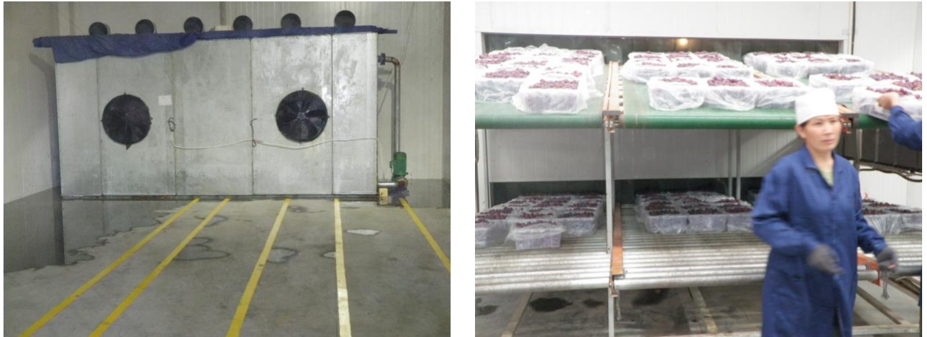
Figure 3.7 Cold room fan-forced pre-cooling (left) and automated pre-cooling unit (right)
