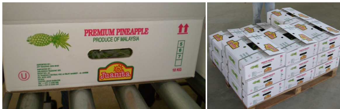
Figure 3.6 10 kg corrugated fibre board boxes currently utilised by the Malaysian pineapple industry for exports to Dubai
