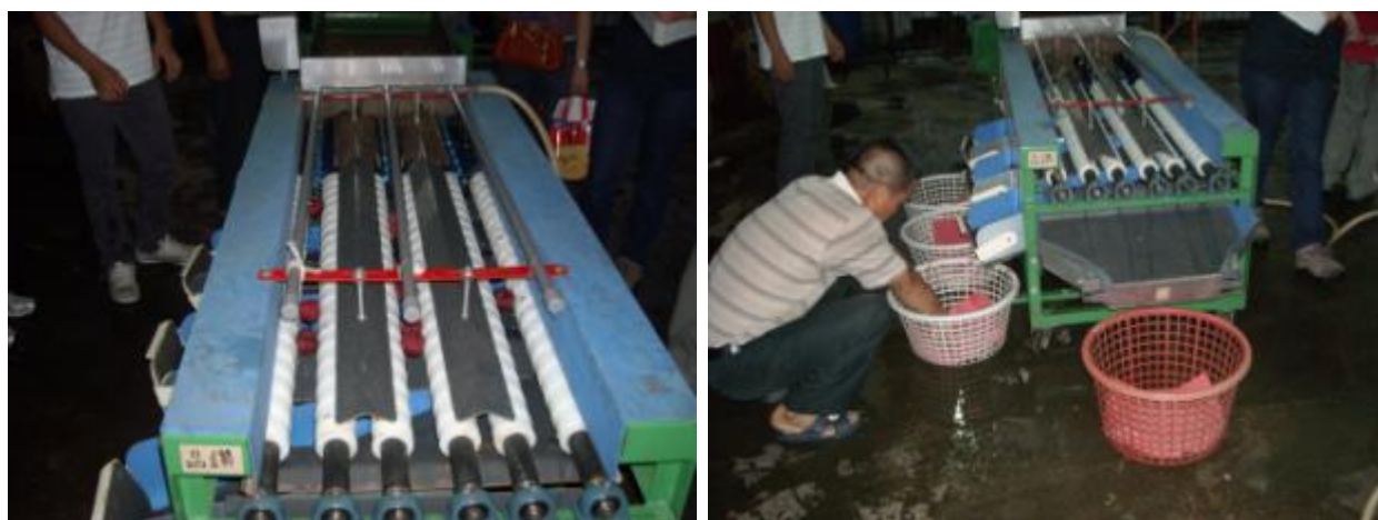
Figure 3.12 Machine used in permanent packing shed for washing and sorting the lychee fruit, Kaohsiung
