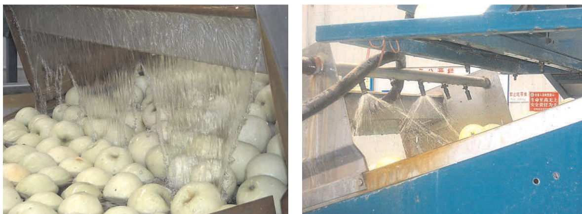
Figure 3.4: Water cleaning facility, showing floating and rinsing of apples
