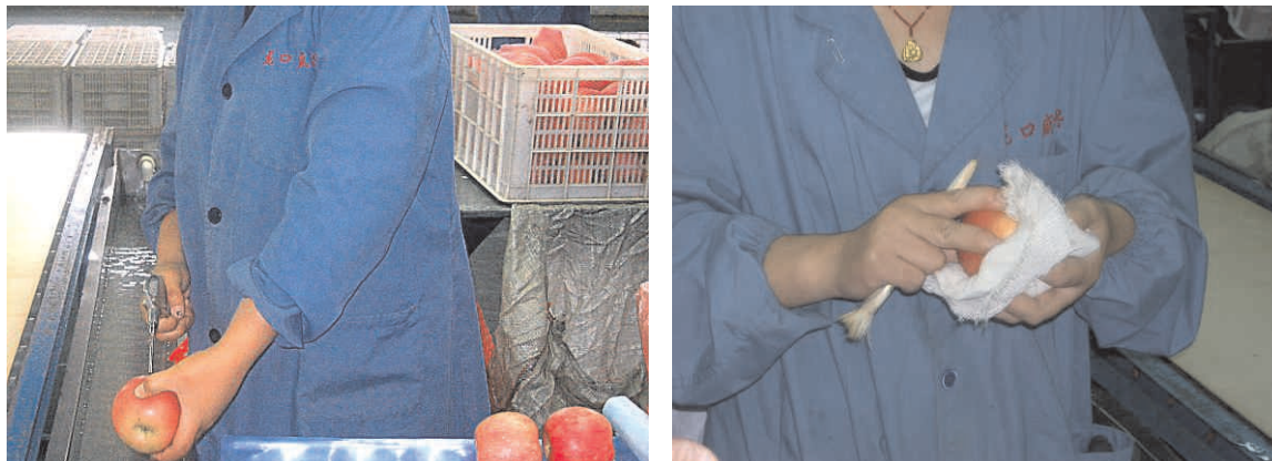
Figure 3.5: Use of pressurised air gun with a water trough (left) and examining and cleaning each fruit (right)
