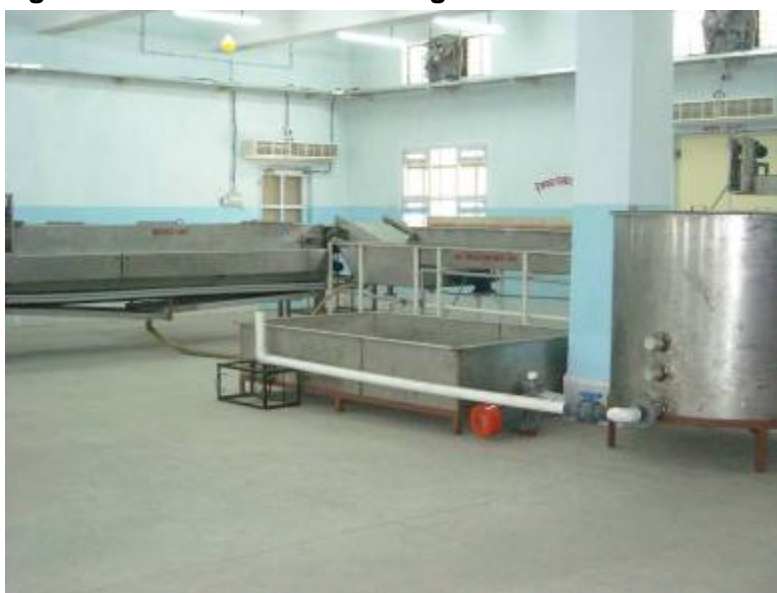
Figure 3.2: Packing house facility for Indian mango fruit, showing hot water fungicidal treatment tank in foreground and washer unit in background
