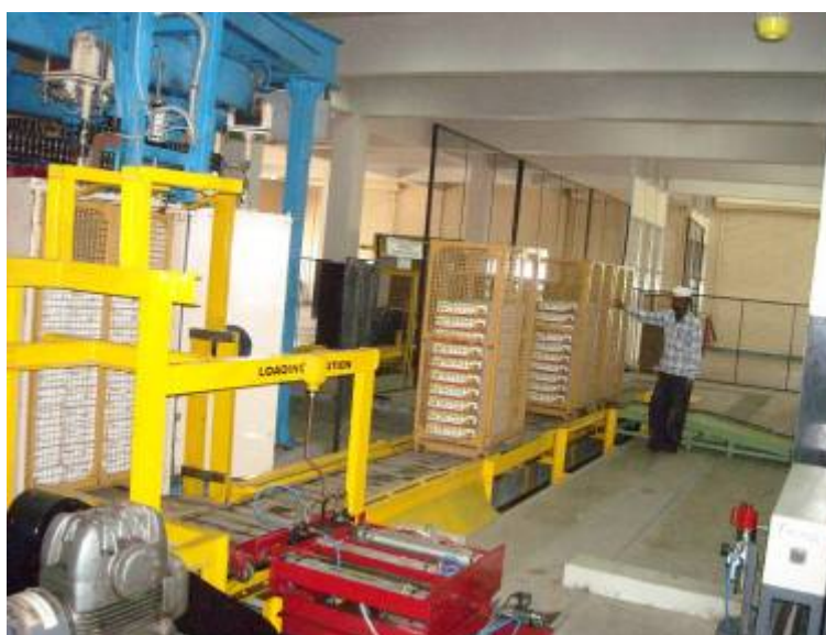
Figure 3.6: At the irradiation facility in Lasalgoan, Maharashtra, mango fruit are loaded into totes ready for treatment
