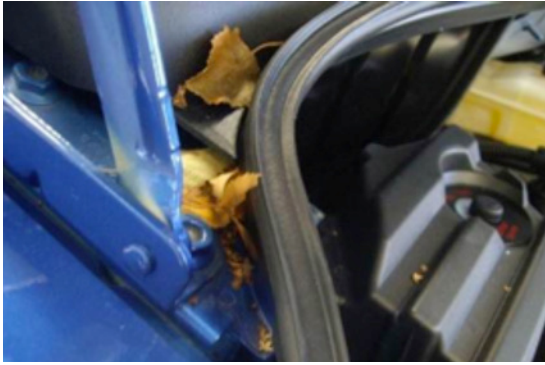
Leaves that have lodged around the plenum chamber area
