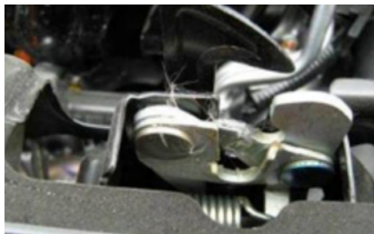
Weed seed in the bonnet latch and other parts of a vehicle
