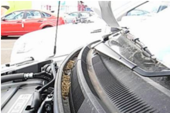
Grain that has lodged around the plenum chamber area
