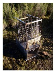
Figure 3 A Mersey Box trap destroyed by a trapped adult wombat attempting to dig its way out. Unlike the trap, the wombat was uninjured, though slightly put out.
