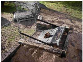
Figure 2 A multi-animal gate trap prototype being developed by Dr Edwards. Multi- or large area animal traps have several potentially attractive characteristics over single animal traps, but further research is needed to identify if they can be used as an effective Alternative to 1080.
