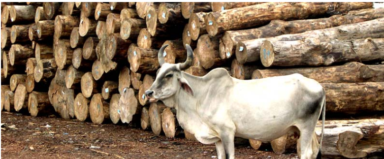
Figure 14 Rough, over-mature radiata pine logs from Australia
