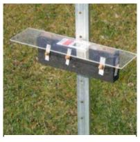
Figure 9 Feratox bait station developed for trials in Tasmania.
