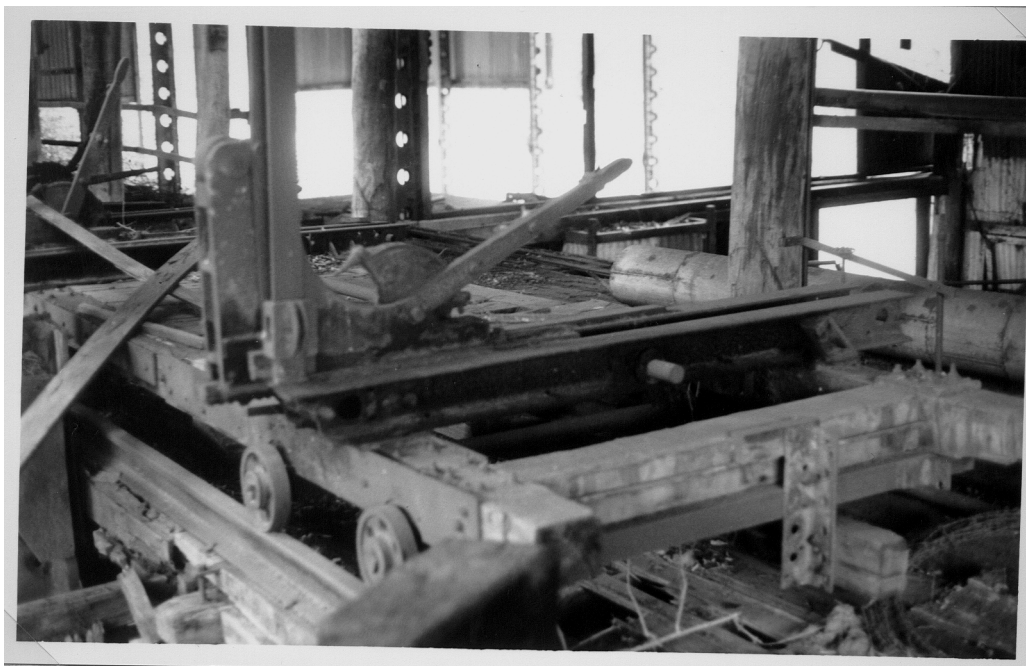
View of log carriage for band saw from western end (shows non-flanged wheels; double-flanged other side)
