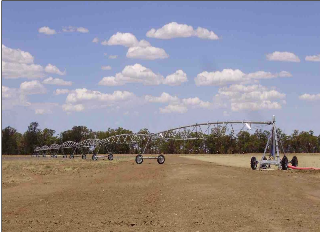
Figure 36: The conversion of 148 ha of border check irrigation to centre pivot irrigation on ‘Old Bundemar’ resulted in water savings about 140 ML/year.
