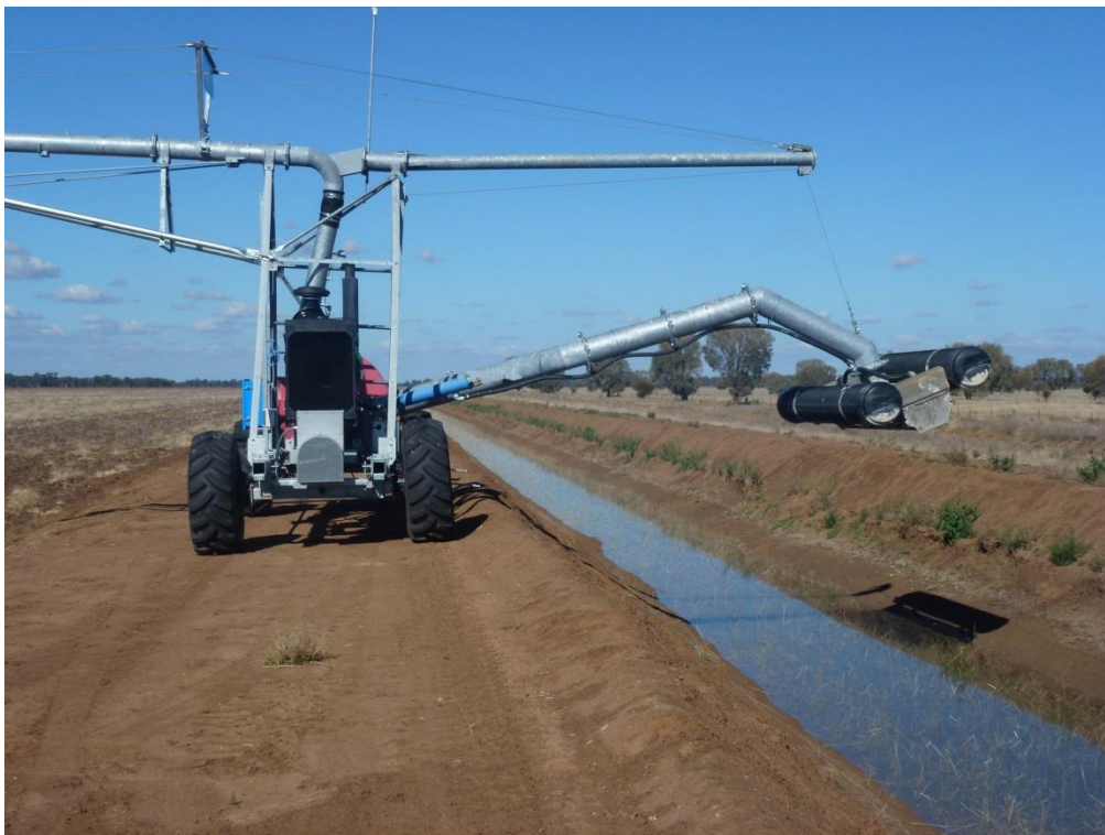
Figure 15: End feed linear move irrigator #1 showing suction cart and supply channel
