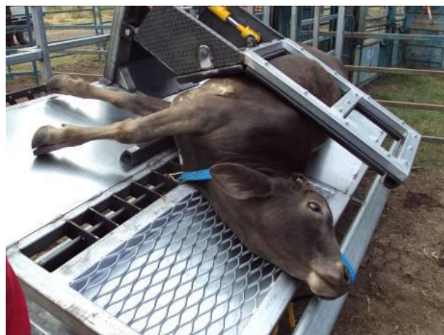
Figure 2 – Testing hydraulic Mark IV restraint box
