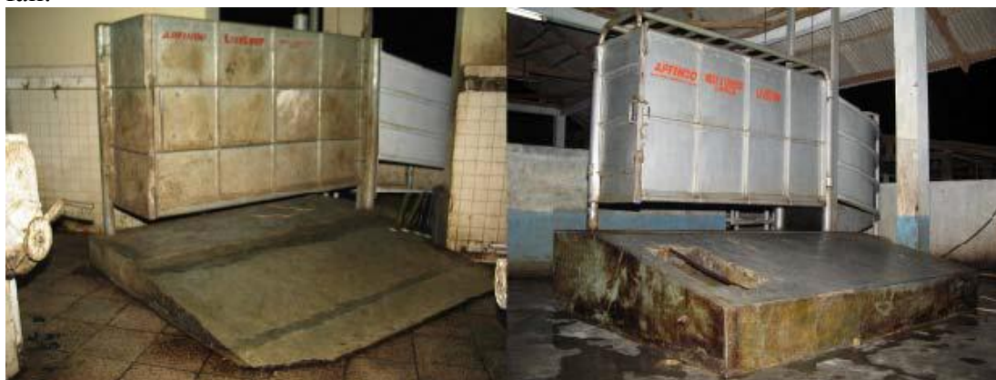
Above: Mark I restraint boxes showing lower plinth height (left figure) and a box with raised plinth (right figure)
